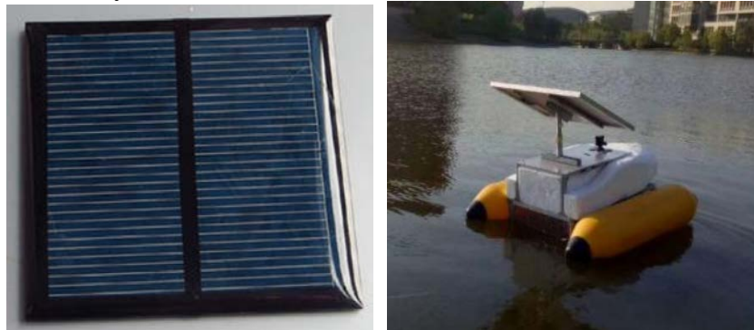
Fig. 1 Miniature solar panel and image figure of the water cleaning robot
